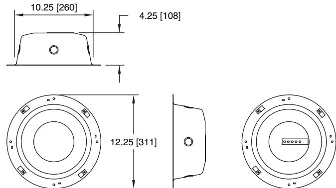
The CT8 loudspeaker can be installed using most industry standard 8" loudspeaker mounting accessories and will retrofit into almost all existing standard 8" diameter loudspeaker openings.
