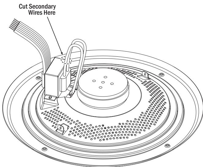
2. Strip  $\frac{1}{4}$ " –  $\frac{1}{2}$ " of insulation from the wires that remain connected to the speaker (not the ones connected to the transformer).
