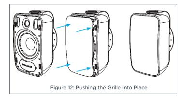
NOTE: To remove the grille, we suggest starting in any one of the four corners using a grille pulling tool (not included). Once the grille is pulled out past the retention clip in one corner, the remainder of the grille can be removed by working your hand around and lightly pulling outward, being careful not to bend the grille skirt. If the grille skirt does become bent during removal, it can be straightened by carefully bending it back into its original shape.
