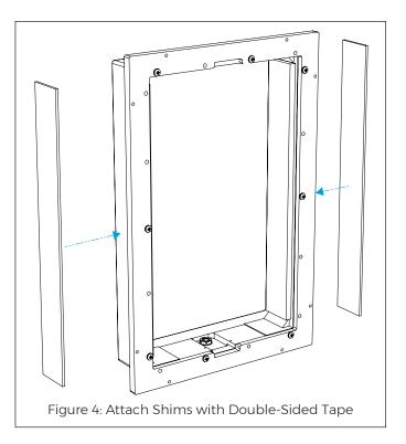
For all other configurations such as 12" OC framing, TJIstyle engineered joists, and/or narrow enclosures, use dimensional lumber, plywood, or other wood shim material to completely fill any gap between the longer sides of the IS Enclosure and construction framing (see Figure 5). This shim material can be either applied to the IS Enclosure or the framing. You may find it easiest to simply frame around all four sides of the enclosure to ensure a snug fit.
