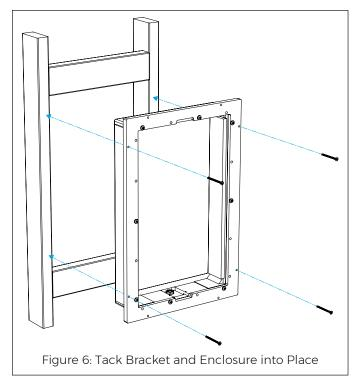
Pre-drill eight pilot holes (four on each side, evenly spaced) through the inside of the IS Enclosure walls, through any shims you have installed, and into the framing (see Figure 7). Avoid drilling the pilot holes near any holes on the face of IS Pre-Construction Bracket. Securely anchor the IS Enclosure to the framing using standard flat head #8 or #10 construction screws (metric equivalent 4–5mm) long enough to drive at least 1" (25mm) into the framing.
