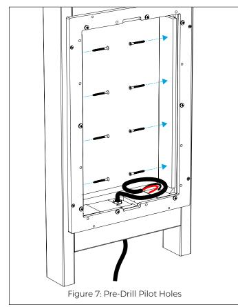
IMPORTANT NOTE FOR NARROW ENCLOSURES: Use the pre-existing holes in the sides of the enclosure to secure to the framing. The screw heads must be countersunk into the IS enclosure walls so that they do not protrude. If you fail to do this, the IS Speaker will not fit. After the screws are installed, you must use gaffer tape or similar to cover all screws and all holes in the walls of the IS Narrow Enclosure to prevent air leaks. Do not skip this step.
