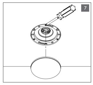
The leveling ring is for fine adjustment. If necessary adjust the magnetic grille leveling ring with a screwdriver and install magnetic grille. See grille painting instructions.
