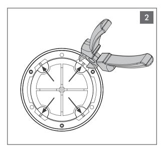
Cut the four tabs on the sanding shield support structure in the speaker bracket. **NOTE: The speaker wire is connected to the zip tie for easy access.**
