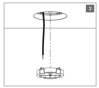
Remove sanding shield support. Remove zip tie from speaker wire.
