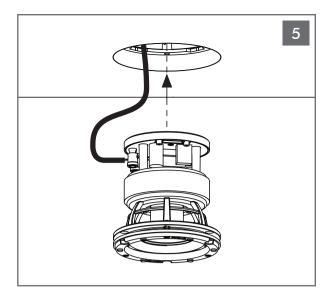
Connect the negative wire to the black spring terminal and the positive wire to the red spring terminal.
