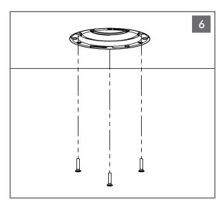
Apply Loctite® to screws and screw speaker to mounting platform.
