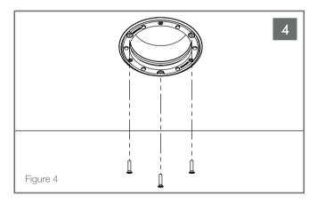
Apply Loctite to the 3 provided screws. Thread the screws through the 3 remaining screw holes of the ASBPC3RS TL and into the brass threaded inserts of the mounting platform. (See Figure 4).
