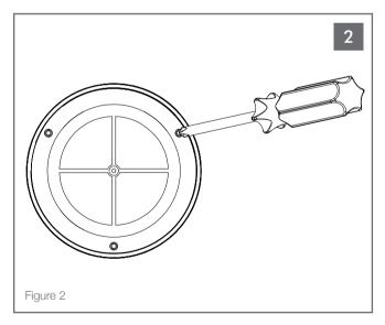
Remove and discard the 3 screws holding the sanding shield support structure using a screwdriver. (See Figure 2).
