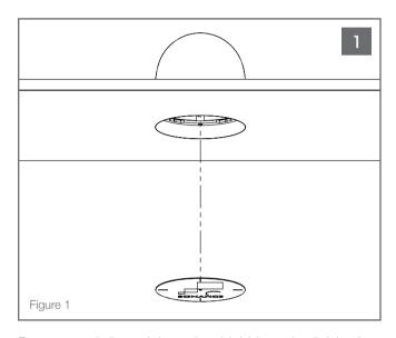
Remove and discard the paint shield from the finished mounting platform. (See Figure 1).
