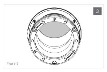
Line up the ASBPC3RS TL with the opening of the mounting platform so that the 3 screws of the ring align with the 3 clearance holes (not threaded) in the mounting platform opening. (See Figure 3).
