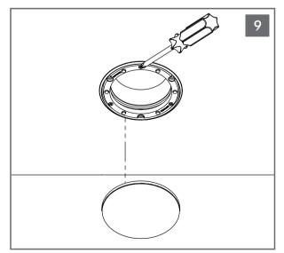
The leveling ring is for fine adjustment. If necessary adjust the magnetic grille leveling ring with a screwdriver so grille installs flush to the ceiling surface. Remove the scrim cloth (for BPS8 Subwoofer applications) and install the grille. **NOTE: See grille painting instructions.**
