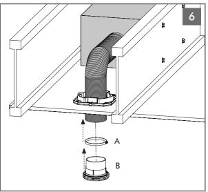
Place the hose clamp (A) around the ASBPS porttube. Slide the port tube over the bandpass connector (B). Orient the port tube on the bandpass connector so the mounting screw locations in the bracket and bandpass connector line up.
