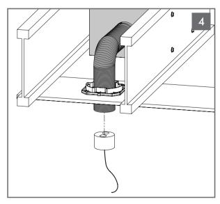
Pull port tube down and expose all extra port tube through speaker opening. Remove foam insert from port tube. Cut and remove extra port tube material, leaving 3 ribs or 1 5/8" (41mm) below ceiling surface.
