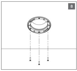
Apply Loctite® to screws and screw bandpass connector to mounting platform.
