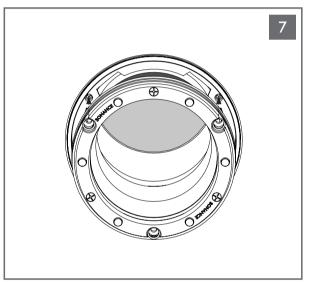
Tighten the hose clamp around the bandpass connector and port tube. The slots in the mounting platform allow clearance for the hose clamp. Orient the hose clamp to go through one of the openings. Place the port tube and connector into the mounting platform.
