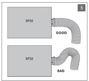
If it is not possible to locate the BPS8 Subwoofer 12" away from the bandpass connector, the extra hose material (up to 8") must be removed. While it is ok to shorten the hose, never extend the hose length.
