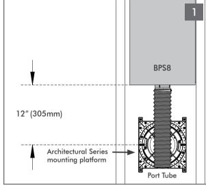
Determine the location for the mounting platform. Ensure there is adequate room for the BPS8 Subwoofer at the location of the platform. The speaker opening must be located 12" (305mm) from the BPS8 Subwoofer to allow the port tube to reach through the platform.
