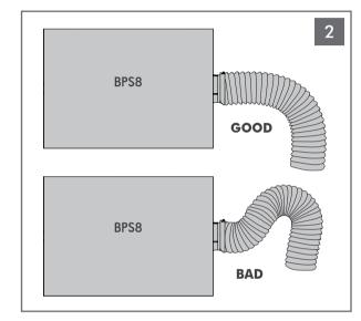
If it is not possible to locate the BPS8 Subwoofer 12" away from the bandpass connector, the extra hose material (up to 8") must be removed. While it is okay to shorten the hose, never extend the hose length.
