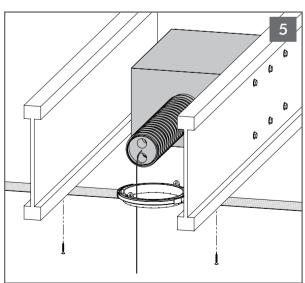
Attach the flex bracket to the joists. The flex bracket must be located within 12" (305mm) of the BPS8 Subwoofer to allow the port tube to reach through the flex bracket opening.
