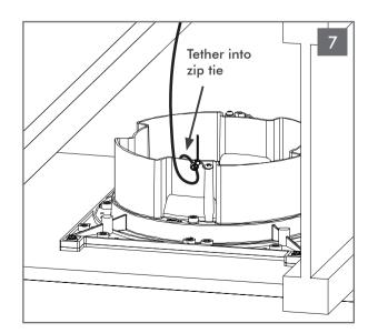
Position end of port tube as close as possible to the back of mounting platform. Loop tether into the anchored zip tie and secure. This process ensures that the bandpass connector is easily attached later and other tradespersons won't infringe on the port tube assembly area.
