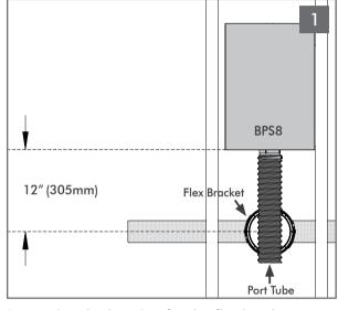
Determine the location for the flex bracket. Ensure there is adequate room for the BPS8 Subwoofer at the location of the flex bracket. The speaker opening must be located 12" (305mm) from the BPS8 to allow the port tube to reach through the flex bracket.
