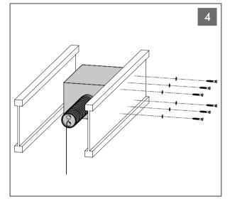
Hold the side of the BPS8 Subwoofer with the rubber damping pad up against the side of the joist and install the six lag screws and washers to secure the BPS8 Subwoofer in place.
