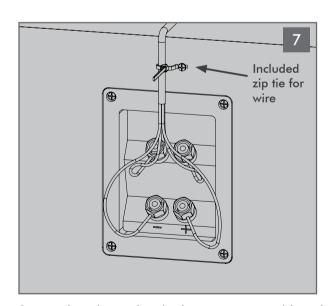
Secure the wire to the zip tie to prevent accidental removal. Attach the four conductor wires to the input terminals. Positive wires to red terminals and negative wires to black terminals. Run a signal test using a 9V battery. **NOTE: Port tube contains foam plug with tether, make sure pressure levels don't expel the foam and tether.**
