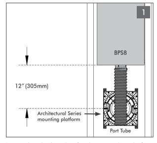
Determine the location for the mounting platform. Ensure there is adequate room for the BPS8 Subwoofer at the location of the platform. The speaker opening must be located 12" (305mm) from the BPS8 Subwoofer to allow the port tube to reach through the platform.
