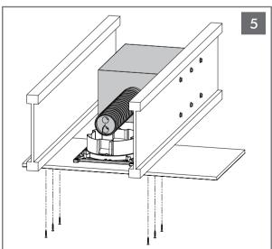
Attach the mounting platform to the joists. For mounting platform installation details visit www.sonance.com/in-wall-in-ceiling/architectural-series/medium-speaker-subwoofer.
