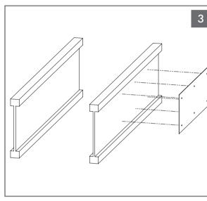
Place the mounting template on the side of the joist and drill six 1/2'' (12.7mm) holes through the joist at the locations shown on the mounting template.
