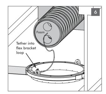
Loop the tether into the flex bracket. Pull the tether all the way until port tube lies firmly on the flex bracket. Tie the tether into a knot. This process ensures that other tradespersons won't infringe on the port tube assembly area.
