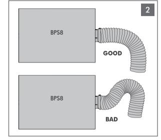
If it is not possible to locate the BPS8 Subwoofer 12" away from the bandpass connector, the extra hose material (up to 8") must be removed. While it is okay to shorten the hose, never extend the hose length.
