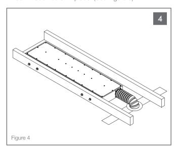
Attach the 3" flex bracket to the 2 x 4 stud or joists in the predetermined location. Check that the mounted distance allows for the port tube to pass through the bracket with at least 4 ribs of the tube exposed. (See Figure 4).
