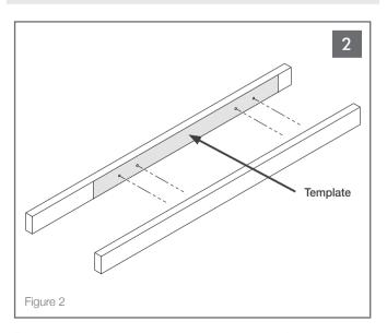
Place the subwoofer mounting template on the side of a  $2 \times 4$  stud or joist and drill four 1/4" (6mm) holes through the locations shown on the mounting template. (See Figure 2).
