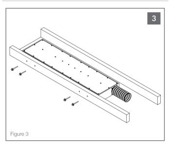
Hold the side of the BPS6 TL Subwoofer with the rubber damping pad up against the side of the 2 x 4 stud and install the four lag screws and washers to secure the BPS6 TL Subwoofer in place. (See Figure 3).
