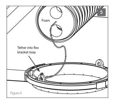
The BPS6 TL ships with a tether inserted into the end of the port tube. Use the tether to guide the port tube into the flex bracket. Loop and pull the tether all the way until port tube lies firmly on the flex bracket. Tie the tether into a knot. This process ensures that other tradespersons won't infringe on the port tube assembly area. (See Figure 5).
