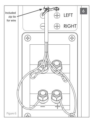
Attach the **four conductor speaker wire** to the input terminals; positive wires to red terminals and negative wires to black terminals. Run a signal test using an amplified program material for at least 60 seconds. Secure the speaker wire to the zip tie attached to the subwoofer cabinet to prevent accidental removal. (See Figure 6).
