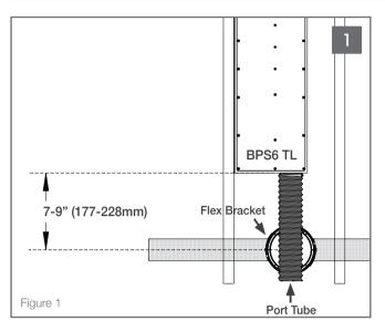
Determine the location of the 3" flex bracket and subwoofer. Ensure there is adequate space to accommodate the subwoofer and port tube within the 2 x 4 stud bay or joists, allowing at least 7-9" from the front edge of the BPS6 TL to the location of the flex bracket opening. (See Figure 1).
