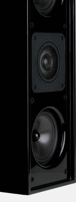
Schance Cinema Living speakers are constructed from the highest quality materials including carbon liber and Richacell® laminated or polypropylene speaker cones, silk dome ferrolluid-cooled tweeters, die-cast aluminum baskets and 3/4" medium density liberboard enclosures.
