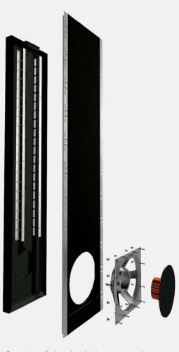
Schance in-wall subwoofer cabinets are constructed from a combination of 1/2" and 1" MDF with extruded aluminum bracing and long-strand fiberglass internal dampening. The floating enclosure design installs into a standard 16" on center stud bay wall, providing the optimum bass response with minimal disturbance in adjoining rooms.
