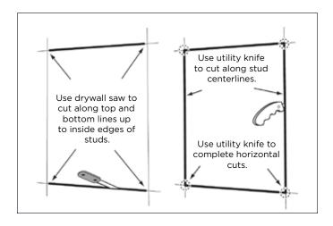
Remove drywall from opening. This should expose only 3/4" (19mm) of each stud/joist or half of the stud/joist surface. Remove any exposed drywall nails or screws.
