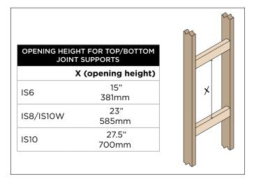
3. Place space saver, preconstruction zip ring bracket, or both in desired speaker location. See page 4 for when to use space savers and zip rings. Space savers are recommended for every new construction project. Zip rings are recommended as a time-saver on very large projects with dozens of invisible speakers.
