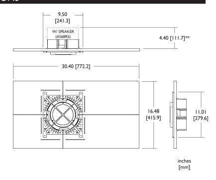
\*\* Depth from back of finish material to back of AS38RS speaker. For depth of subwoofer and accessory options, see dimension drawings
