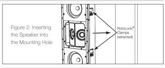
NOTE: THE ROTOLOCK® SYSTEM CAN ACCOMMODATE A WALL MATERIAL THICKNESS OF 1 1/4" (32MM). WITH THE TOGGLE FOOT CAP REMOVED, THE SYSTEM CAN ACCOMMODATE A WALL MATERIAL THICKNESS OF 1 1/8" (28MM).
