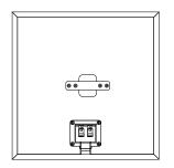
Includes back plate compatible with third party seismic retention hardware.
