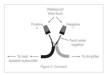
NOTE: SONANCE STRONGLY RECOMMENDS THE USE OF 14/4 DIRECT BURIAL WIRE FOR DISTANCES UP TO 200 FEET AND 12/4 DIRECT BURIAL FOR LONGER RUNS. KEEP WIRES AS SHORT AS POSSIBLE TO MINIMIZE RESISTIVE WIRE LOSSES.
