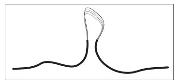
4. Use a wire tie to keep the wire loop intact and act as a strain relief.
