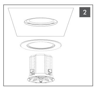
Connect Speaker wires as per In-Ceiling Speaker Installation Manual then insert the speaker through the Retro Ring and then slide up into the hole in the ceiling and through the C-bracket.
