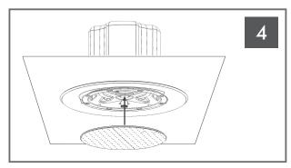
After the speaker is installed, and the transformer tap and tweeter angle adjustments are made as per the In-Ceiling Speaker Installation Manual, the grille can be installed. The grille is held in place by several small, powerful magnets on the speaker frame. Place the grille against the speaker and the magnets will hold it firmly in place.
