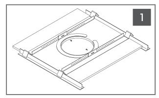
Insert the two tile support rails and C-bracket through the hole you have cut, placing them as shown. Using the two screws that are supplied, screw the C-bracket to the tile support rails as shown.
