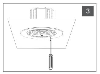
Tighten the four screws on the front of the baffle. The Roto-Lock Clamps will rotate into position automatically and begin clamping. When you notice resistance on the four screws, the speaker has been clamped successfully. The flange is designed to flex and conform to any small imperfections in the ceiling surface.
