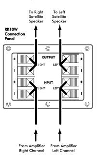
4. After you have made the previous connections, connect the wires to your amplifier. Double-check that you connected all of the wires properly (amplifier '+' to speaker '+; amplifier '-' to speaker '-') at all of the connections.
