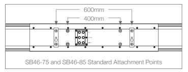
To hang key hole wall mount use only #10 - #12 pan head or flat head screws (not supplied). The screws must be firmly attached to the studs to support the weight of the soundbar. Align the screw heads into the large round portion of the key hole and gently slide into place.
