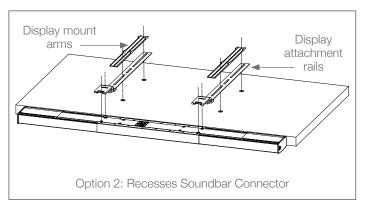
Position the soundbar as close to display as possible. Firmly fasten B. screws with I. washers to connect soundbar to the soundbar connectors.
