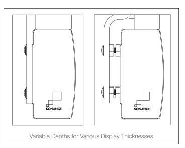
NOTE: IF THE SPACERS ARE NOT USED, THE FRONT SURFACE OF THE DISPLAY WILL BE IN LINE WITH THE FRONT RADIUS OF THE SOUNDBAR GRILLE. THIS IS DEPENDENT ON THE DISPLAY THICKNESS AND INSTALLATION PREFERENCE.
