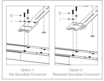
Secure the wall bracket and attachment rails to the display using spacers and screws supplied with the wall mount or E. and F. screws with H. and I. washers (depending on the size of the display's threaded Inserts. E. and H. are M6; F. and I. are M8). Hardware will vary. It is recommended to keep spacers and hardware provided with display or display mount. Refer to your display manual for the proper torque to be applied to the screws.
