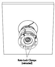
14. Tighten the screws on the front of the speaker baffle. The Roto-Lock toggle feet will automatically rotate into position and begin clamping the speaker. When you notice resistance on the screws the speaker has been clamped successfully.
