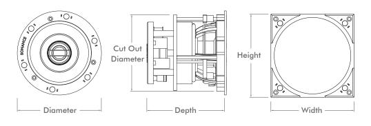
**VPBPC3R** Diameter: 4 5/16" (109mm) Cut Out Diameter: 3 15/16" (99mm) Depth: 3 1/2" (89mm)
