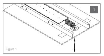
Inspect the installed BPS6 TL flex bracket location for the BPS6 TL port tube and clamp ring. Pull the port tube through the flex bracket to ensure that at least 4 ribs or 2 1/2" (63.5mm) of the tube are exposed through the opening. (See Figure 1).
