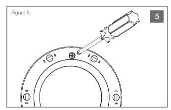
Once the VPBPC3R TL face is flush with the surface, use a screwdriver to tighten the two RotoLock clamp screws until the clamps grip the back of the surface and secure the VPBPC3R TL into place. (See Figure 5).
