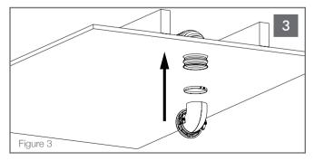
Loosen the clamp ring on the port tube and slide the VPBPC3R TL into the end of the exposed tube. Tighten the hose clamp to secure the port tube to the VPBPC3R TL. (See Figure 3).
