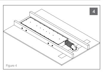
Feed the tube and attached VPBPC3R TL back into the flex bracket hole, rotating ¼ turn clockwise as necessary to relieve any tube resistance within the wall or ceiling. (See Figure 4).
