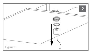
Remove and discard the foam plug and tether from within the port tube. (See Figure 2).
